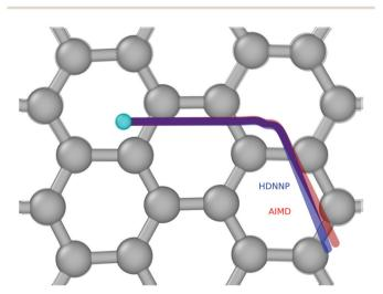
Fig. 5 The same two trajectories as in Fig. 4-AIMD (red) and HDNN-PES (blue). The H-atom's initial position is shown as a cyan colored ball. The divergence between the two trajectories is due to residual error in the NN fit to the DFT data. A "side view" of the trajectories can be found in the ESI.†
