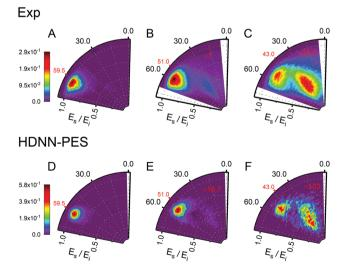
Fig. 7 Comparing theory with experiment for D-scattering from graphene at  $E_i = 1.9$  eV. Experimental distribution are shown in panels (A-C) along with theoretical distribution found from MD simulations using the HDNN-PES (D-F). The number of trajectories used for the plots are shown in Table S2 in the ESI.†
