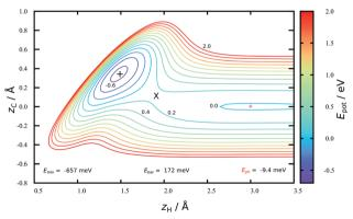
Fig. 2 A cut through the HDNN-PES in the vicinity of the minimum energy path to chemisorption. The H atom is constrained to lie directly above a C-atom.  $z_H$  and  $z_C$  indicate the distance of H and C, respectively, from the plane of the graphene sheet. The physisorption (+) and chemisorption (+) minima have depths of 9 and 657 meV, respectively. The barrier to chemisorption (x) has a height of 172 meV.
