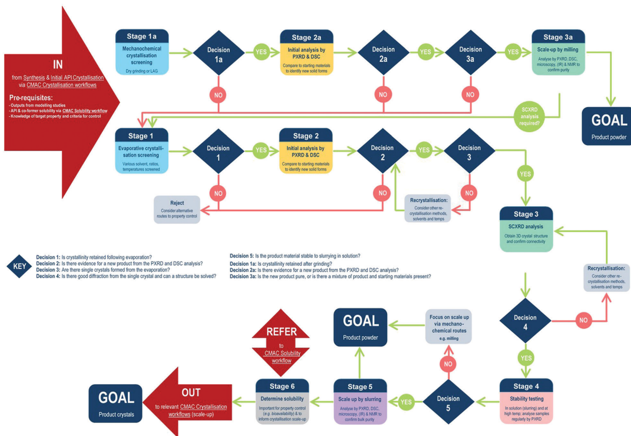
Fig. 1 CMAC multicomponent (MC) material screening workflow. The workflow is driven by the decision points as indicated in the text; these capture the key elements indicating if the co-crystallisation process is likely to have value. Light blue squares indicate points at which the CCDC software tools are implemented. Decision 1: is crystallinity retained following evaporation?; Decision 2: is there evidence for a new product from the PXRD and DSC analysis?; Decision 3: are there single crystals formed from the evaporation?; Decision 4: is there good diffraction from the single crystal and can a structure be solved?; Decision 5: is the product material stable to slurring in solution?; Decision 1a: is crystallinity retained after grinding?; Decision 2a: is there evidence for a new product from the PXRD and DSC analysis?; Decision 3a: is the new product pure, or is there a mixture of product and starting materials present?
