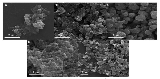
Fig. 1 SEM images of the synthesized ZIF-8-GA with A) 2.0, B) 10.0, C) 15.0 and D) 20.0 mg ml<sup>-1</sup> of GA and (E) ZIF-8 without GA in a total volume of 10.0 ml and linker/metal molar ratio of 4.0.
