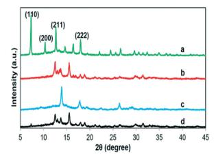
Fig. 4 The XRD patterns of ZIF-8-GA in linker/metal molar ratios of a) 20.0 b) 10.0 c) 4.0 in the presence of GA (15.0 mg ml<sup>-1</sup> in a total volume of 10.0 ml) and d) 20.0 in the absence of GA.
