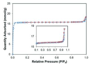
Fig. 6 Nitrogen adsorption-desorption isotherms of ZIF-8-GA.
