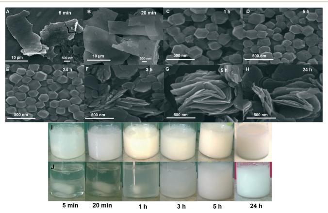
Fig. 3 SEM images and photographs of synthesis solution at linker metal molar ratio of 20.0/1.0/2800 as a function of time (A–E and I) in the presence and (F–H and J) absence of 15.0 mg ml<sup>-1</sup> GA.
