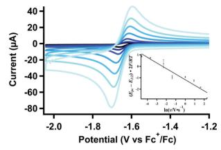
Fig. 1 Variable scan-rate CVs (0.025–10 V s<sup>-1</sup>) of  $[Pt(depe)_2](PF_6)_2$  (1) (1.06 mM) with  $CH_2(TBD)_2 \cdot HPF_6$  (5.00 mM) and (b) linear plot for the change in cathodic peak potential used for calculating  $k_{obs,H^+}$ . Additional data used for calculation shown in Fig. S1 and S2 (ESI†).
