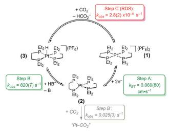
Scheme 1 Proposed catalytic cycle and corresponding rates of reactions for electrocatalytic CO<sub>2</sub> reduction to HCO<sub>2</sub> by [Pt(depe)<sub>2</sub>](PF<sub>6</sub>)<sub>2</sub> (1). Conditions: 5 mM 1, 100 mM CH<sub>2</sub>(TBD)<sub>2</sub>·HPF<sub>6</sub>, 1 atm CO<sub>2</sub>.
