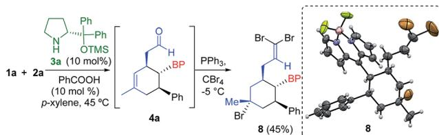
Scheme 2 Derivatization of compound **4a** and X-ray analysis of compound **8**.
