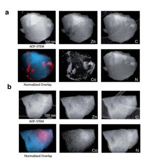
Fig. 5 (a) ADF STEM image, EDS elemental maps for C, N, Zn and Co signals, and Zn (blue) and Co (red) component map overlay of (ZIF-67)(ZIF-62)(20/80), (b) ADF STEM image of a shard of  $a_g[(ZIF-67)_{0.2}(ZIF-62)_{0.8}]$  and corresponding C, N, Zn and Co EDS elemental maps, and an overlay map of Zn (blue) and Co (red) components.
