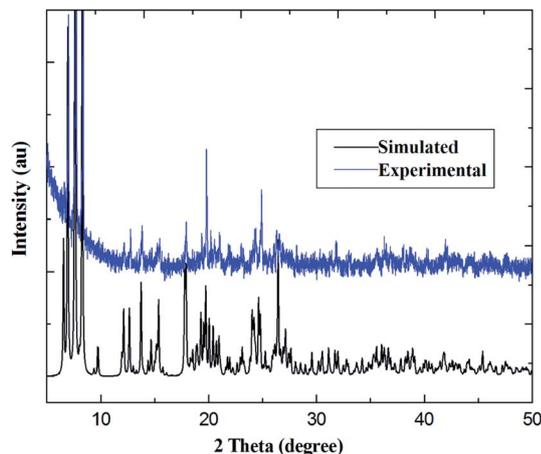
Fig. 3 Comparison of simulated and experimental PXRD patterns for Pr(III) compound 1.
