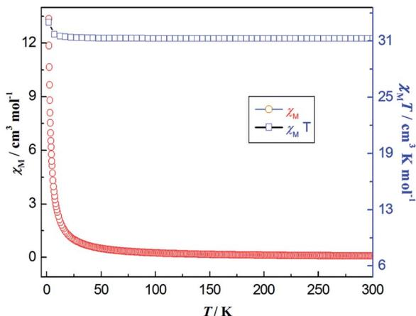
Fig. 14 Thermal variation (temperature dependence) of  $\chi_M T$  ( $\square$ ) and  $\chi_M$  ( $\circ$ ) versus  $T$  for coordination polymer 7 under the DC magnetic field of 1000 Oe.
