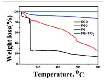
Fig. 5 TGA analysis of SGO, FGO, FG and FG-HTiO<sub>2</sub> samples.
