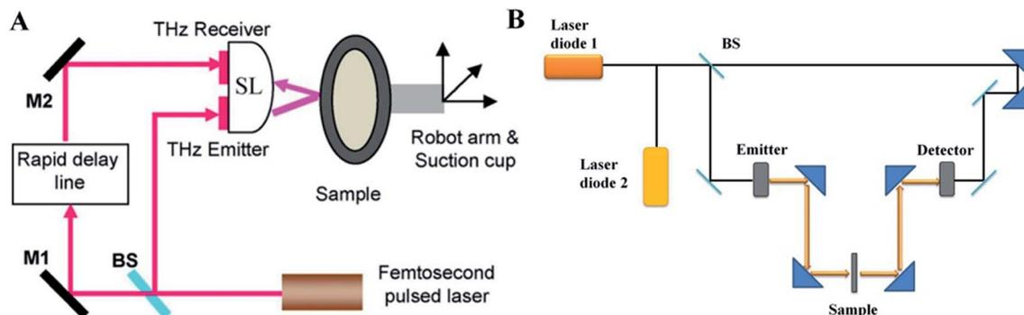
Fig. 2 Schematic illustration of THz imaging system. (A) TPI reflection system. (B) The CW THz imaging system in transmission geometry.
