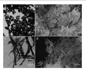
Fig. 2 TEM and SEM images of the prepared Fe<sub>3</sub>O<sub>4</sub> nanoparticles (a and b) and  $Fe_3O_4$ -Ag nanocomposite (c and d).
