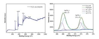
Fig. 6 XPS profiles of the Fe<sub>3</sub>O<sub>4</sub>-Ag nanocomposite (a) and the deconvolution of Ag peaks (b).
