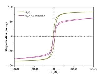
Fig. 5 Magnetization hysteresis loops of as-prepared Fe<sub>3</sub>O<sub>4</sub> nanoparticles and Fe<sub>3</sub>O<sub>4</sub>-Aq nanocomposite.
