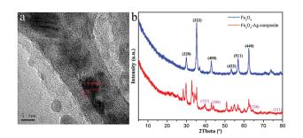
Fig. 4 HRTEM image of Ag nanowires (a) and XRD patterns of the Fe<sub>3</sub>O<sub>4</sub>-Ag nanocomposite (b).
