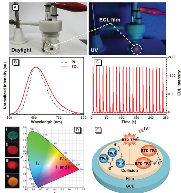
**Fig. 3** (A) Digital photos of the experimental setup after the ECL experiment under daylight and UV illumination. (B) Normalized ECL and PL spectra of the **BTD-TPA** films. Excitation: 460 nm. (C) ECL stability of the **BTD-TPA** films. (D) ECL photos of **BTD-Ph** (I), **BTD-TPA** (II), and **BTD-NPA** (III) in DCM solution, the **BTD-TPA** film (IV), and CIE chromaticity coordinates of their ECL spectra. (E) Proposed ECL mechanism of **BTD-TPA** films.
