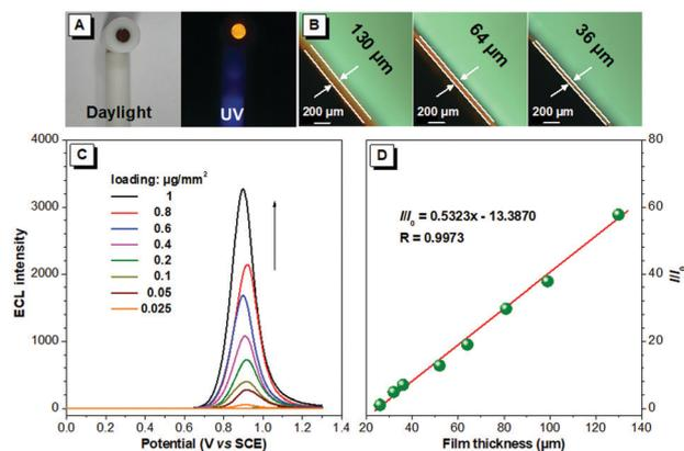
**Fig. 4** (A) Digital photos of **BTD-TPA** film under daylight and UV illumination. (B) Optical microscope images of **BTD-TPA** films with different thicknesses. (C) ECL intensity of **BTD-TPA** films with various loadings. (D) Plot of relative ECL intensity ( $I/I_0$ ) versus the different thickness of **BTD-TPA** films;  $I_0$  denotes the ECL emission intensity of **BTD-TPA** film with a thickness of 26 μm.
