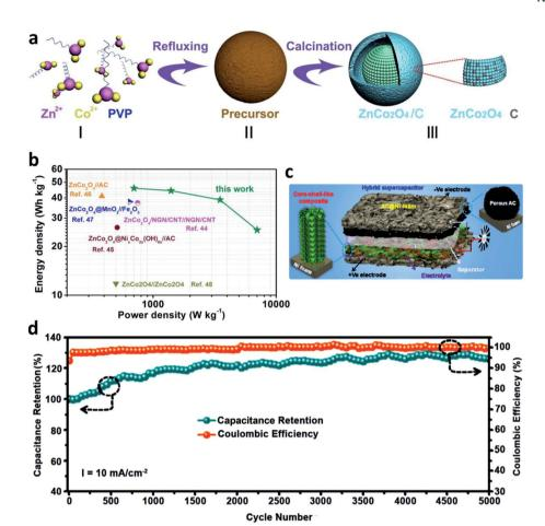
Fig. 4 (a) Scheme of the synthesis a yolk-shell structure  $ZnCo_2O_4$  material, (b) Ragone plots of AACSDs (modified from ref. 85, copyright permission from the Royal Society of Chemistry); (c) illustration for the preparation process and (d) cycling stability of core-shell-like  $NiO_6Co_3O_4$ - $NiO_7FN/Ni$  foam (modified from ref. 88, copyright permission from Elsevier).
