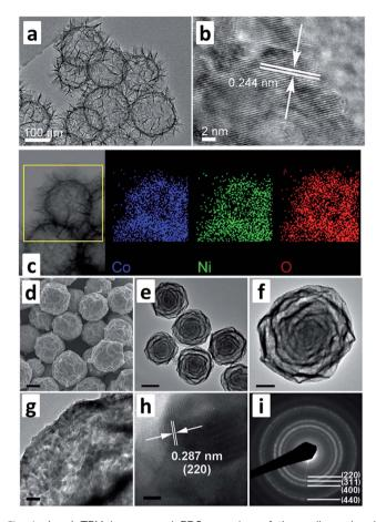
Fig. 1 (a–c) TEM images and EDS mapping of three dimensional NiCo $_2$ O $_4$  nanospheres, (d–i) SEM and TEM images of seven-layered Ni–Co oxide spheres derived from MOF (modified from ref. 32 and 33, copyright permission from Elsevier and Wiley-VCH, respectively).
