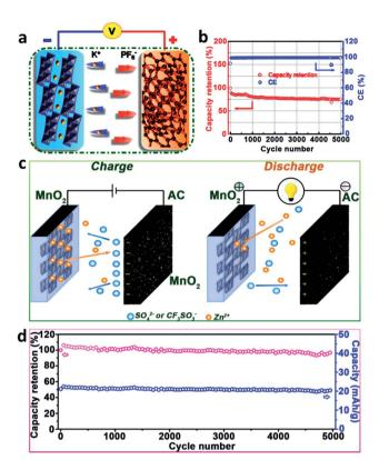
Fig. 9 (a) Schematic and (b) long-term cycling stability at the current density of 1 A  $\rm g^{-1}$  of a NGC//KTO KIHSCD (modified from ref. 125, copyright permission from the American Chemical Society); (c) schematic illustration and (d) cycling stability of a designed MnO<sub>2</sub>//AC ZIHSCD (modified from ref. 126, copyright permission from Elsevier).
