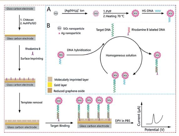
Fig. 19 Schematic illustration of a MIP-based electrochemical DNA biosensor for the determination of breast cancer susceptibility gene (BRCA-1) amplified by  $SiO_2@Ag$ . Insets of (A) and (B) show the preparation process of  $SiO_2@Ag/DNA$  and homogeneous DNA hybridization. Reproduced with permission from ref. 154. Copyright 2018, Elsevier.
