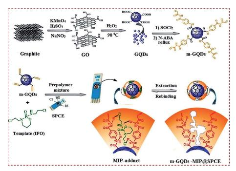
Fig. 7 (a) Schematic illustration for the preparation of monomeric graphene quantum dots (m-GQDs) and fabrication of screen-printed carbon electrode (SPCE) modified with m-GQD-MIP. Reproduced with permission from ref. 88. Copyright 2017, Elsevier.
