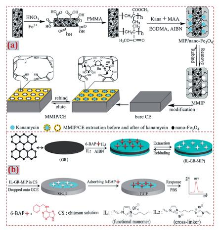
Fig. 8 (a) Schematic of the preparation process of magnetism imprinted electrochemical sensor based on MWCNTs decorated on Fe<sub>3</sub>O<sub>4</sub> NPs. Reproduced with permission from ref. 103. Copyright 2015, Elsevier. (b) Schematic illustration for the synthesis of IL-GR-MIP composite dropped on GCE and the detection process for the electrochemical sensor. Reproduced with permission from ref. 131. Copyright 2018, Elsevier.
