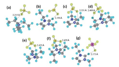
Fig. 15 Ion-pair structures in vacuo optimized using HF/6-31 + G(d,p), (a)  $TEA^+BF_4^-$ , (b)  $EMI^+BF_4^-$ , (c)  $TMI^+BF_4^-$ , (d)  $AMN^+BF_4^-$ , (e)  $TMIN^+BF_4^-$ , (f)  $TEMIN^+BF_4^-$ , and (g)  $EMI^+PF_6^-$ . This figure has been adapted from ref. 152 with permission from The Electrochemical Society.
