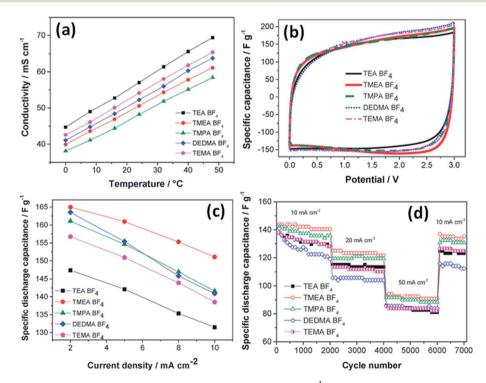
Fig. 13 (a) Conductivity values vs. temperature, (b) CV in various electrolytes at 2 mV  $s^{-1}$ , (c) capacitance values at low currents, and (d) cycle life tests. This figure has been adapted from ref. 121 with permission from the Royal Society of Chemistry
