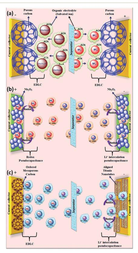
Fig. 12 Graphical representation of reaction mechanism between organic electrolytes and various electrodes for (a) EDLC (b) pseudocapacitor (c) hybrid supercapacitor.
