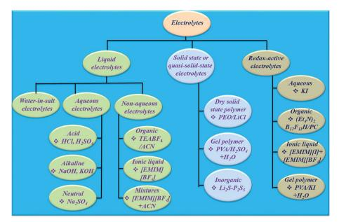
Fig. 4 Classification of electrolytes for electrochemical supercapacitors.
