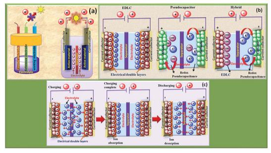
Fig. 1 (a) Schematics of the three-electrode configuration and two-electrode configuration, (b) type of supercapacitors: EDLC, pseudocapacitor and hybrid, (c) charge storage mechanism in EDLCs, ion absorption and desorption on the surface.
