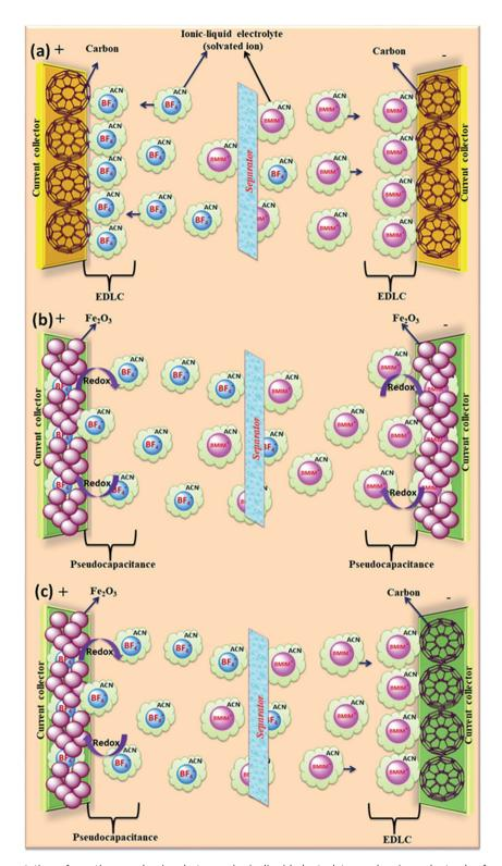
Fig. 16 Graphical representation of reaction mechanism between ionic-liquid electrolytes and various electrodes for (a) EDLC (b) pseudocapacitor (c) hybrid supercapacitor.
