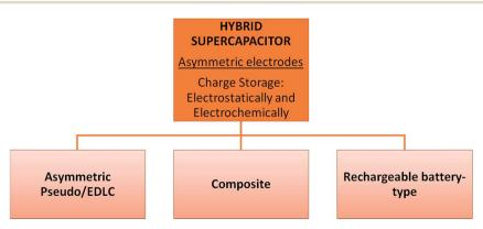
Fig. 4 Classification of hybrid supercapacitors into three types according to their design or working mechanism.
