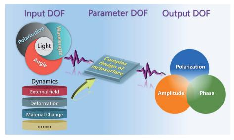
Fig. 1 Schematic of DOF in metasurface designs. The input DOF includes the properties of incident light and working conditions. The output DOF corresponds to the properties of re-radiated light. By controlling the parameter DOF of the complex metasurface, the desired properties and functionalities of output signals can be realized.
