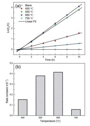
Fig. 14 (a) Time dependent MB concentration showing the photocatalytic decomposition kinetic behaviour of the NT powders obtained at various annealing temperatures; (b) the photocatalytic rate constant. Reproduced from ref. 14 with permission from the Springer Publishing group under Creative Commons Attribution 4.0 International License.
