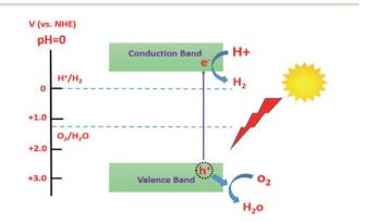
Fig. 9 Semiconductor requirements for solar water splitting
