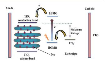
Fig. 8 Schematic diagram of a DSSC using TNTP as an anode.
