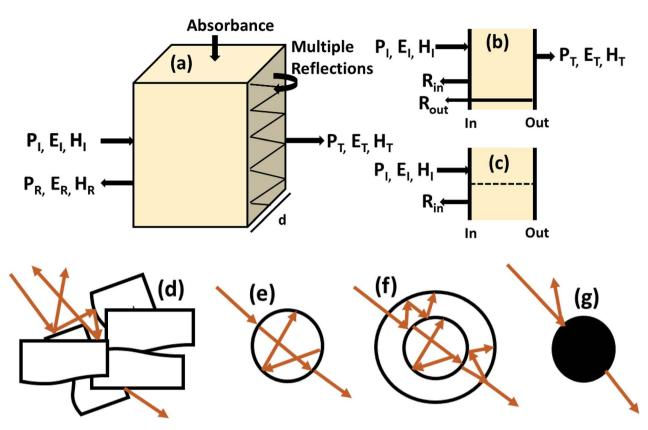
Fig. 2 (a) Schematic diagram of incident, reflected and transmitted power and electro-magnetic field intensities when an EM wave is incident on a 3D material; (b and c) sources of reflection in a thin sample (input and output interfaces,  $R_{in}$  and  $R_{out}$ ) and in a thick sample; (d-g) multiple reflections in the case of a porous structure, a hollow structure, a multiple shell structure and a solid sphere.
