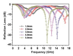
**Fig. 18** Reflection loss of GNpFe $_3$ O $_4$ @ZnO composites with thickness 1–5 mm  $^{181}$  – reproduced by permission of the Royal Society of Chemistry.
