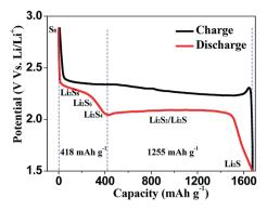
The typical charge-discharge curve of lithium-sulfur batteries.
