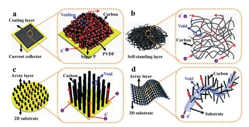
Fig. 6 The schematic illustration of the comparison between the electrode with binder and several typical binder-free electrodes. (a) Electrode with binder; (b) self-standing electrode; (c) array structure on a 2D substrate electrode; (d) array structure on a 3D substrate electrode.
