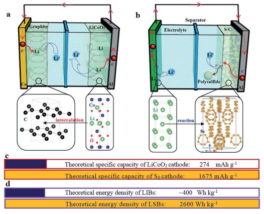
Fig. 2 A schematic illustration of the working principles of a graphite/LiCoO<sub>2</sub> lithium-ion battery (a) and a lithium-sulfur battery (b). The crystal structure of graphite, LiCoO<sub>2</sub>, Li metal and sulfur is also given at the corresponding positions. (c) The comparison of theoretical specific capacities of the LiCoO<sub>2</sub> and  $S_8$  cathodes. (d) The comparison of theoretical energy densities of LIBs and LSBs.
