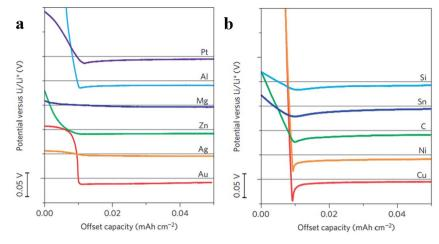
Fig. 15 (a) Voltage profiles of various materials with some solubility in Li during Li deposition at a current density of  $10 \,\mu\text{A cm}^{-2}$ ; (b) shifted voltage profiles of various materials with negligible solubility in Li during Li deposition at a current density of  $10 \,\mu\text{A cm}^{-2}$ ; the horizontal gray lines show  $0 \,\text{V}$  versus Li in (a) and (b). (a–c) Reproduced with permission.<sup>123</sup> Copyright 2016, Nature Publishing Group.
