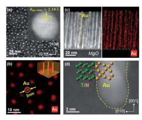
Fig. 2 Detailed microstructure analysis of low-density Au-TiN thin film grown on MgO. (a) Plan view STEM image and high resolution of Au nanopillar top projection (inset image). (b) Plan view energy-dispersive X-ray spectroscopy (EDS) mapping of Au nanopillars, where Au is mapped as red color, inset is the illustration of low density Au-TiN hybrid platform. (c) Cross-sectional STEM and EDS mapping. (d) Cross-section HRSTEM showing the Au-TiN interface, and its atomic model.
