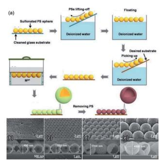
Fig. 2 (a) Schematic illustration of the formation process of ordered metal oxide macroporous hollow spherical arrays. (b–e) Fabricated Fe $_2$ O $_3$  hollow spherical arrays with different aperture sizes by using 500, 1000, 2000, and 5000 nm PS spherical templates. Reproduced with permission.<sup>48</sup> Copyright 2017, Elsevier Ltd.
