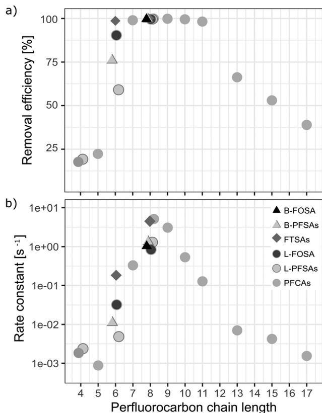
Fig. 4 a) Maximum removal efficiencies [%] after 8 h of ozonation and b) second order reaction rate constants [ $s^{-1}$ ] for all analyzed PFASs of varying perfluorocarbon chain lengths and functional groups in the pilot-scale ozonation treatment. Rate constants were calculated according to the second order rate law described by Atkins *et al.*<sup>50</sup>
