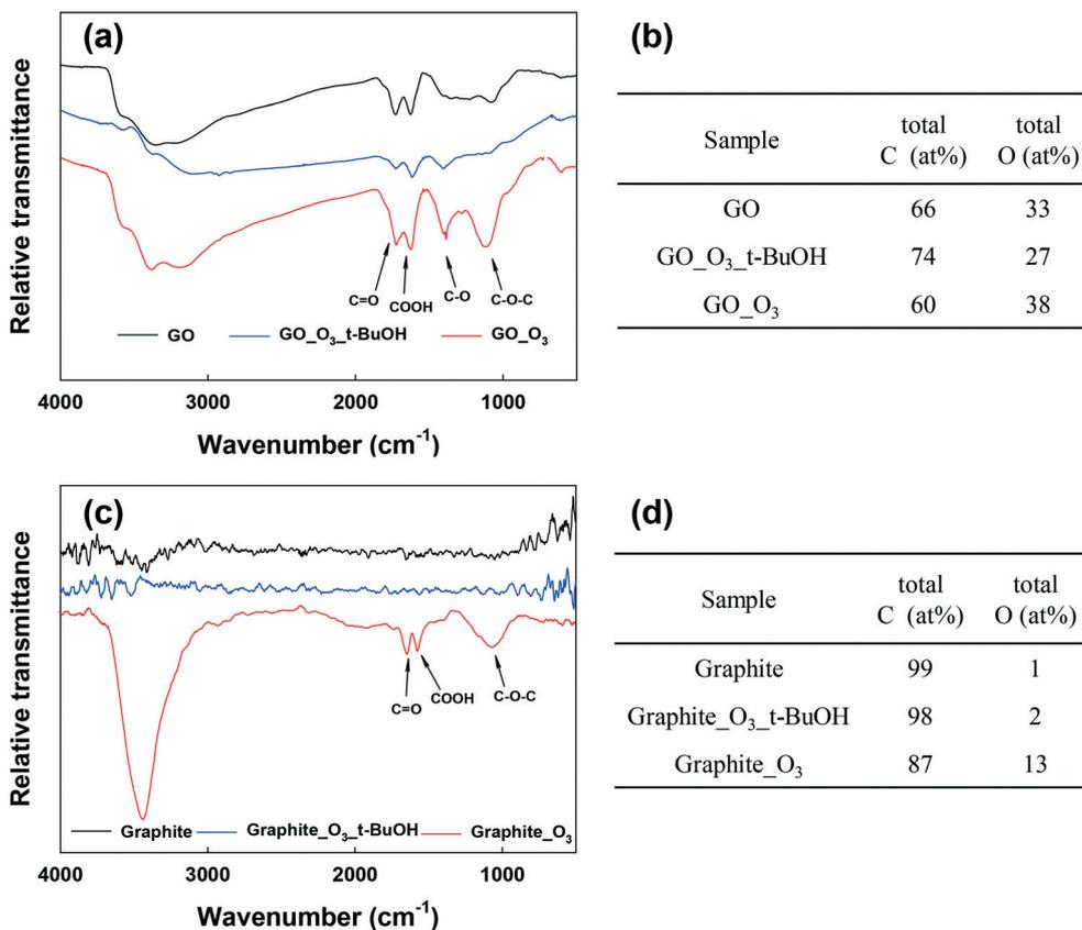
Fig. 4 (a) FTIR spectra of GO, GO\_O<sub>3</sub> with t-BuOH and GO\_O<sub>3</sub>. (b) C and O ratio of GO, GO\_O<sub>3</sub> and GO\_O<sub>3</sub> with t-BuOH obtained from XPS analysis. (c) FTIR spectra of graphite, Graphite\_O<sub>3</sub> with t-BuOH and Graphite\_O<sub>3</sub>. (d) C and O ratio of graphite, Graphite\_O<sub>3</sub> and Graphite\_O<sub>3</sub> with t-BuOH obtained from XPS analysis.
