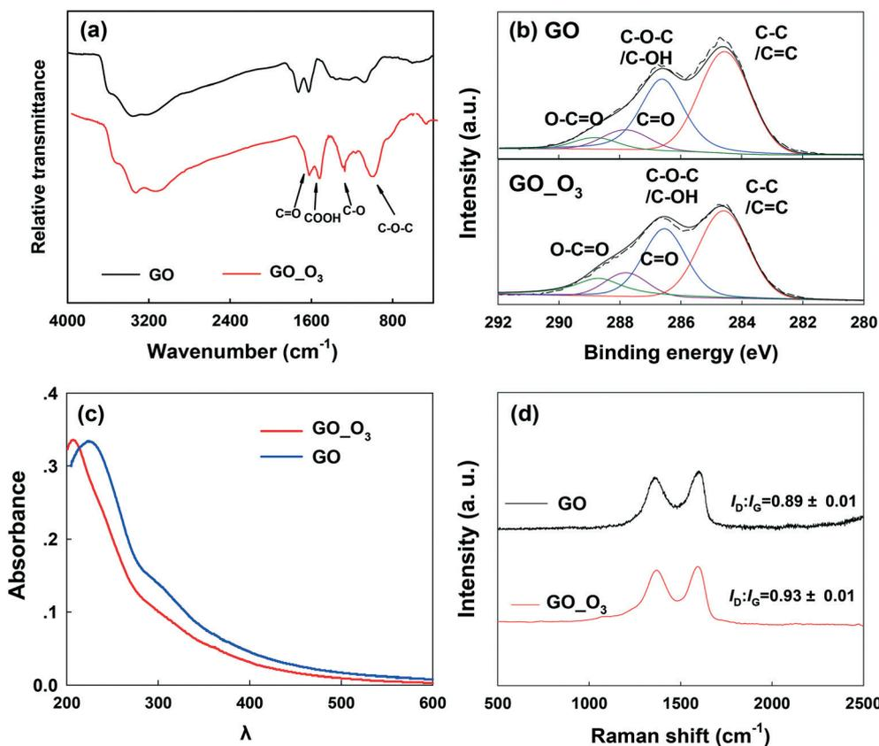
**Fig. 2** (a) Fourier transform infrared (FTIR) spectroscopy, (b) X-ray photoelectron spectroscopy (XPS), (c) UV-vis spectrophotometry, and (d) Raman spectroscopy of pristine GO and  $O_3$ -treated GO ( $GO_{O_3}$ ).
