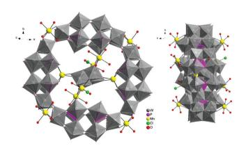
Fig. 2 Combined polyhedral/ball-and-stick representation. Front and side views of the structure of  $Mn_{10}W_4$ - $P_8W_{48}$ . Alkali metal cations are omitted for clarity.
