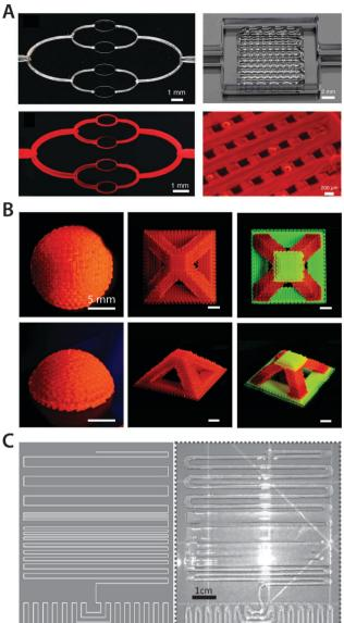
Fig. 21 Direct ink writing 3D printing of hydrogels. (A) 3D printed hydrogels with micro-scale vascular networks. Adopted with permission from ref. 208. Copyright 2014 Wiley-VCH. (B) Multi-material high resolution 3D printing of hydrogels into various geometries. Reproduced with permission from ref. 211. Copyright 2018 Wiley-VCH. (C) 3D printed ionically conductive hydrogel circuits on silicone elastomer substrate. Adopted with permission from ref. 209. Copyright 2017 Wiley-VCH.
