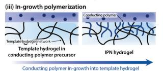
Fig. 15 Various preparation routes toward conducting polymer IPN hydrogels. IPN hydrogels are typically prepared through three major approaches: (i) direct mixing between conducting polymers and the template hydrogel precursor, (ii) in situ polymerization of conducting polymers within the hydrogel template, and (iii) in-growth polymerization of conducting polymers into the hydrogel template.
