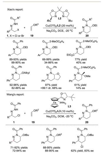
Scheme 8 Copper complex catalyzed IEDDA reaction of azoalkene with
