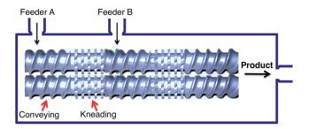
Fig. 2 A schematic twin screw extrusion setup.
