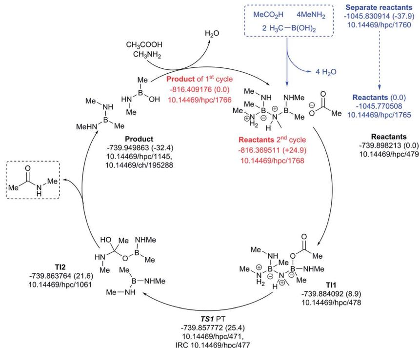
Fig. 12 Catalytic cycle involving four amines (data<sup>29</sup> sub-collection DOI: 10.14469/hpc/1728; the labels have the same meaning as in Fig. 9). All DOIs in this figure are available as clickable links (final paginated PDF only).
