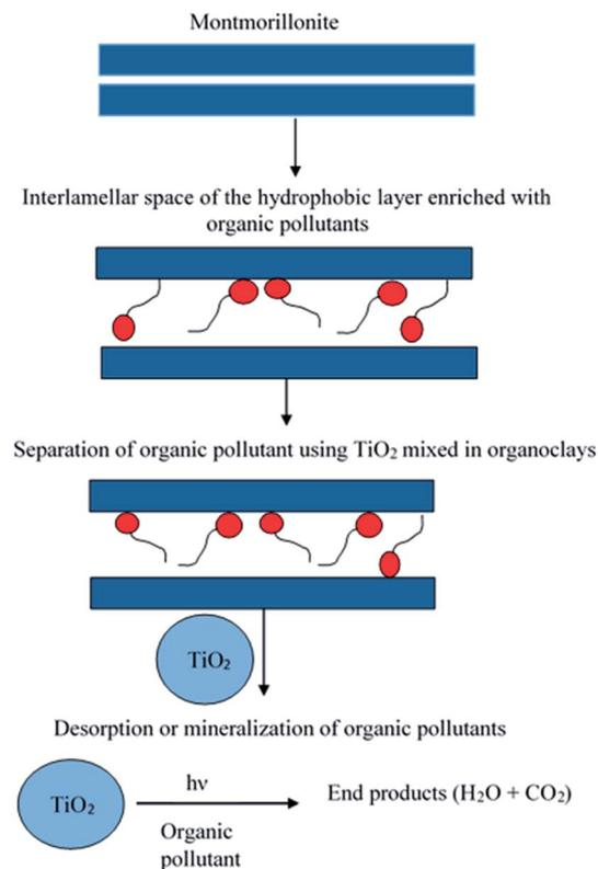
Fig. 8 Scheme for the photocatalytic regeneration of dye pollutants using  $\text{TiO}_2$ . This figure has been adapted/reproduced from ref. 179 with permission from Taylor & Francis.
