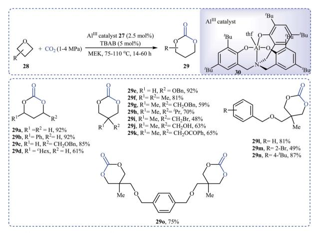
Scheme 13 Al(III)-catalyzed coupling of oxetanes 28 with CO<sub>2</sub> reported by Kleij.
