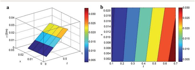
Fig. 7 Dependences of conductivity on "f" and "x" parameters at average values of other factors: (a) 3D and (b) contour plots.
