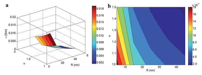
Roles of "R" and "u" parameters in the conductivity of nanocomposites at average levels of other parameters: (a) 3D and (b) contour plots.
