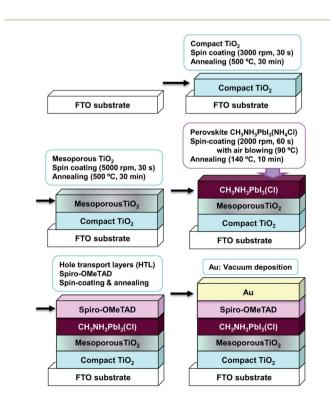
Fig. 1 Schematic illustration of the process used to fabricate the  $CH_3NH_3PbI_3(Cl)$  photovoltaic cells.
