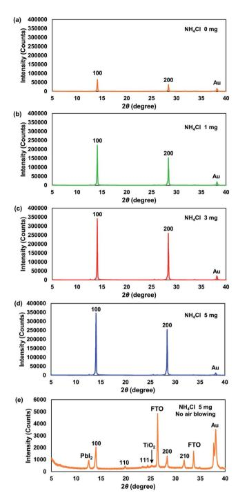
Fig. 7 XRD patterns of  $CH_3NH_3Pbl_3(Cl)$  cells containing (a) 0 mg, (b) 1 mg, (c) 3 mg, and (d) 5 mg of  $NH_4Cl$ , and (e) XRD pattern of the  $CH_3NH_3Pbl_3(Cl)$  cell containing 5 mg of  $NH_4Cl$  without air blowing.
