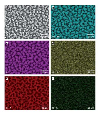
Fig. 5 (a) SEM image of the  $CH_3NH_3Pbl_3(Cl)$  cell without  $NH_4Cl$ , and corresponding elemental mapping images of the (b) Pb M line, (c) I L line, (d) Cl K line, (e) C K line, and (f) N K line.
