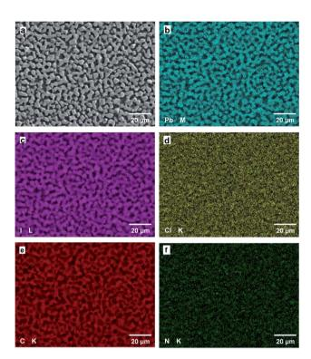
Fig. 6 (a) SEM image of the  $CH_3NH_3PbI_3(Cl)$  cell containing 5 mg of  $NH_4Cl$ , and corresponding elemental mapping images of the (b) Pb M line, (c) I L line, (d) Cl K line, (e) C K line, and (f) N K line.
