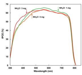
Fig. 3 IPCE spectra of  $CH_3NH_3PbI_3(CI)$  solar cells with and without  $NH_4CI$ .
