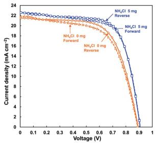
Fig. 2 J-V characteristics of  $CH_3NH_3PbI_3(Cl)$  solar cells with and without  $NH_4Cl$ .
