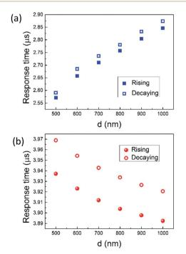
Fig. 10 Rising and decaying time as function of d in the structure without air trench (a) and with air trench (b)
