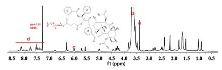
Fig. 1 <sup>1</sup>H NMR spectra of PTX-PEG
