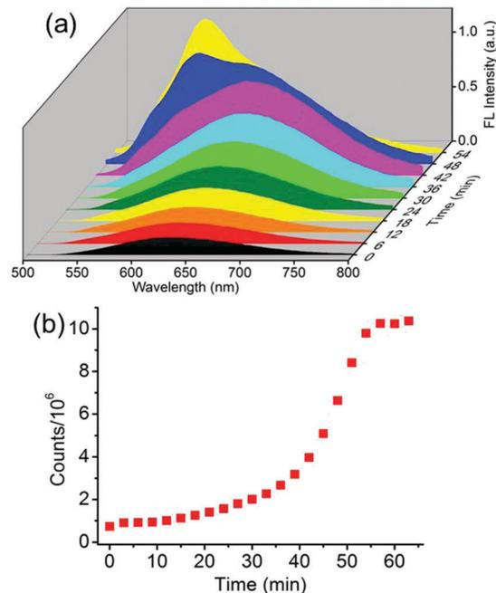
Fig. 3 (a) The emission changes during the morphological transition from nanospheres to nanorods by adding CTAB (1.5 mg mL<sup>-1</sup>) to the aqueous dispersion of nanospheres. (b) The time-dependent emission intensities monitored at  $\lambda = 580$  nm during the process of nanosphere–nanorod transition.
