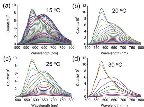
Fig. 4 The emission changes at different temperatures during the formation of the nanorods. (a) 15 °C, (b) 20 °C, (c) 25 °C, and (d) 30 °C.  $C_{\text{CTAB}} = 1.0$  mg mL<sup>-1</sup>. The spectra were recorded every 3 min.
