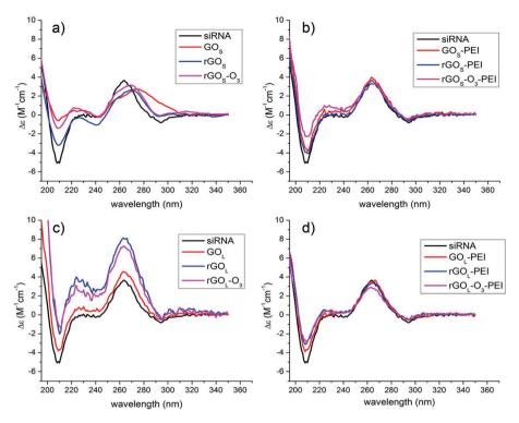
Fig. 4 CD spectra of siRNA after incubation and filtration with a series of: (a) GO<sub>S</sub>, (b) GO<sub>S</sub>-PEI, (c) GO<sub>L</sub>, and (d) GO<sub>L</sub>-PEI, respectively.
