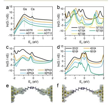
Fig. 3 Calculated room-temperature conductance of (a) ADT, (b) X[T3]X, (c) X[Ph]X, and (d) X[V]X vs. Fermi energy for alkyl chains with different numbers of  $CH_2$  groups.  $E_F = 0$  corresponds to the DFT-predicted Fermi energy. LDOS at -0.15 eV (e) showing Cs, and at -1.11 eV (f) showing Gs
