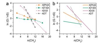
Fig. 4 Comparison of experimental (a) and calculated (b) natural logarithm of conductance versus the number of methylene units in the side chains for the four series of molecular wires considered in this study. See Fig. S1-S10 (ESI‡) for individual histograms.
