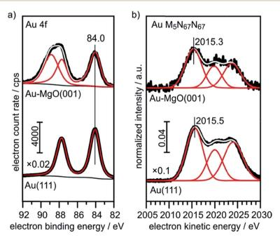
Fig. 6  $\,$  XPS and X-ray excited Auger reference spectra of Au(111) and 0.4 ML Au on 30 ML MgO(001)/Ag(001).
