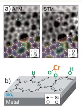
Fig. 1 (a) Atomic force microscope (AFM) and STM images of the amorphous bilayer silica film grown on Ru(0001), that are superimposed with a silica network. (b) Schematic view of a planar model system for the Phillips catalyst, where Cr species are anchored onto an atomically flat hydroxylated silicate film (reprinted with permission from ref. 43. Copyright (2017) Elsevier).
