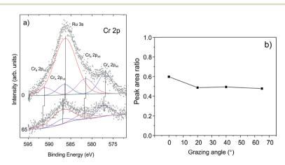
Fig. 3 (a) The deconvoluted Cr 2p signals in XP spectra and (b) the peak area ratios of Cr 2p and Si 2p signals measured as a function of electron emissions.
