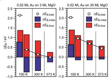
Fig. 8 Graphical representation of the  $E_{\rm B}$ -shifts derived from  $\Delta\beta$  measurements for 0.02 ML Au on 3 ML MgO(001)/Ag(001) (left) and 0.2 ML Au on 30 ML MgO(001)/Ag(001) (right) with reference to Au(111) from Table 1.
