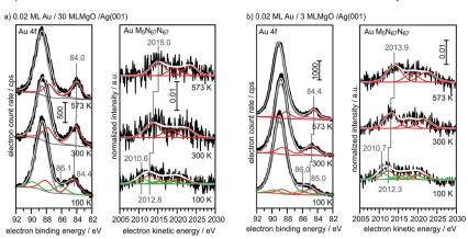
Fig. 7 XPS and X-ray excited Auger spectra of 0.02 ML Au/30 ML MgO (a) and 0.02 ML Au/3 ML MgO (b) for different annealing temperatures (bottom: 100 K; middle: 300 K; top: 573 K).
