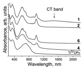
Fig. 14 Spectra of pristine Ti<sup>IV</sup>O(Pc<sup>2-</sup>) and selected salts 1, 2, 4 and 6 in the UV-visible-NIR ranges in KBr pellets. Pellets for the salts were prepared under anaerobic conditions.
