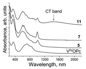
Fig. 15 Spectra of pristine V<sup>IV</sup>O(Pc<sup>2-</sup>) and selected salts 5, 7 and 11 in the UV-visible-NIR ranges in KBr pellets. Pellets for the salts were prepared under anaerobic conditions.
