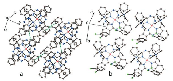
Fig. 2 (a) View of the phthalocyanine layer composed of the π-stacking [{Ti<sup>IV</sup>O(Pc<sup>-3-</sup>)}<sup>-1</sup>]<sub>2</sub> dimers in 1.<sup>12</sup> Short van der Waals C,N···C,N contacts are shown by green dashed lines. (b) Projection of the  $Et_4N^+-C_6H_4Cl_2$  layer on the phthalocyanine layer. Only one phthalocyanine from the dimer is shown (bonds are shown in grey).
