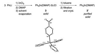
Scheme 1 Preparation of Ph<sub>3</sub>In(DMAP) (3') and ORTEP drawing (showing 40% probability displacement ellipsoids) of the crystal structure of Ph<sub>3</sub>In(DMAP). The hydrogen atoms are omitted for clarity. CCDC 1579360.†
