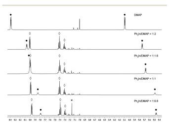
Fig. 1 Ph<sub>3</sub>In(DMAP) stoichiometry experiments. • DMAP.  $\Diamond$  Ph<sub>3</sub>In.  $\times$  Benzene (resulting from Ph<sub>3</sub>In decomposition).
