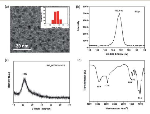
Fig. 1 (a)TEM image of SiNPs, inset shows size distribution of SiNPs by DLS measurement. (b) Characteristics toward Si2p in SiNPs by XPS. (c) XRD pattern and (d) FT-IR spectrum of SiNPs.
