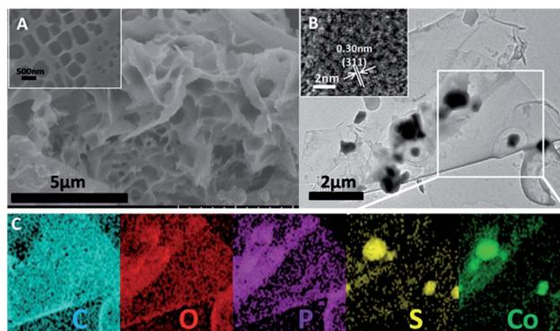
Fig. 1 (A) and (B) SEM and TEM images of  $\text{Co}_9\text{S}_8$ @NPC-10. The insets in (A) and (B) are the corresponding high magnification SEM and high resolution TEM images. (C) Corresponding elemental mapping analysis of the selected area from (B).
