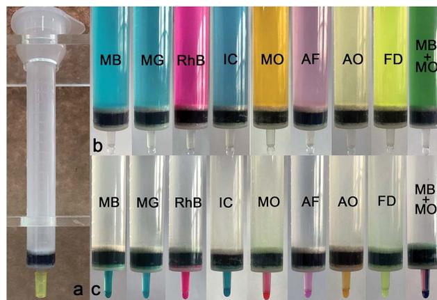
**Fig. 5** (a) Chromatography column is filled with PCN-222 microcrystalline 200 mg. (b) Eight cationic or anionic dyes or MB–MO mixture are loaded on the column. (c) Dyes are washed off by 0.1 M HCl/methanol or saturated NaCl/DMF.
