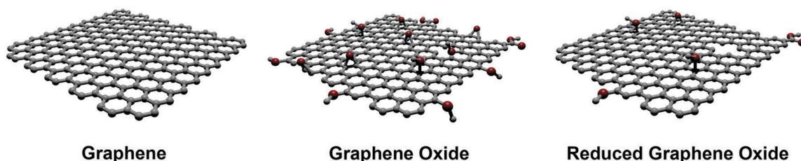
Fig. 1 Molecular structures of graphene, GO and rGO.
