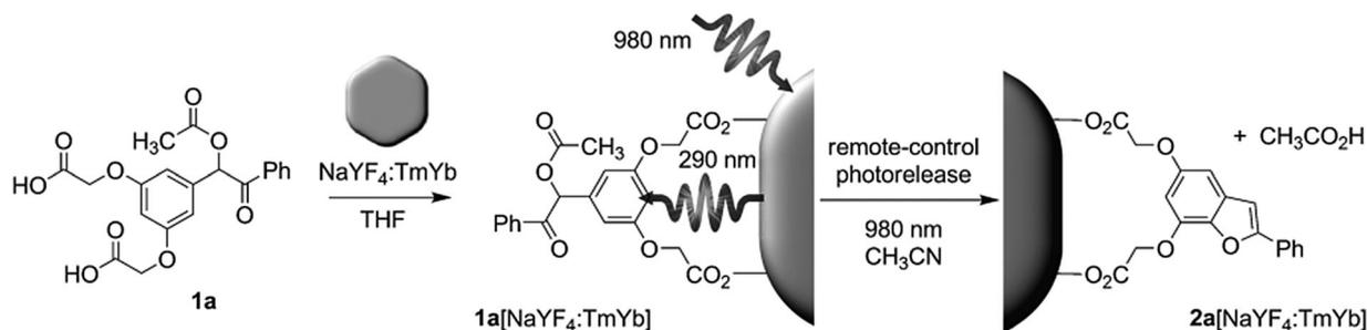
Fig. 5 UCNP-assisted photolysis at surfaces of UCNPs. Decoration of UCNPs with 3',5'-di(carboxymethoxy)benzoin cage **1a** produces the remote-control release system (**1a**[NaYF<sub>4</sub>:TmYb]), which can be triggered by indirect irradiation with NIR light to generate **2a**[NaYF<sub>4</sub>:TmYb] and release a carboxylic acid. Reproduced with permission.<sup>71</sup> Copyright 2010, Wiley-VCH Verlag GmbH & Co. KGaA.
