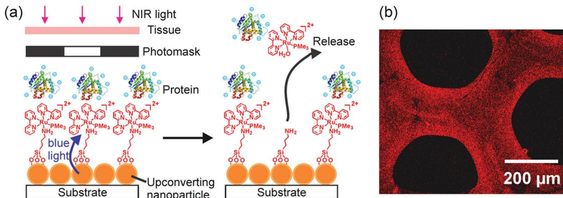
**Fig. 11** (a) Schematic of photon upconversion lithography for the patterning of proteins. Polyethylene glycol, which is co-grafted with Ru complexes on the UCNPs, is not shown for clarity. (b) Confocal laser scanning microscopy image of a protein pattern fabricated using photon upconversion lithography. Adapted with permission.<sup>81</sup> Copyright 2015, Wiley-VCH Verlag GmbH & Co. KGaA.
