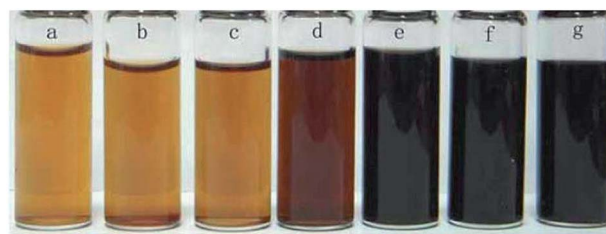
Fig. 11 Photographs of GO suspension with concentration of 0.56 mg mL -1 (a–f) under different conditions. (a) GO aqueous suspension after microwave treatment for 1 min, (b) GO suspension in DMAC/H 2 O (6 : 1), (c–f) GO suspension in DMAC/H 2 O (6 : 1) after microwave treatment for 1, 2, 3, and 10 min (2 min × 5 times), respectively, (g) re-dispersed of the dried graphene into pure DMAC with concentration of 1.0 mg mL -1 . 128 Reprinted (adapted) with permission from ref. 128. Copyright © 2010 Elsevier B. V. All rights reserved.
