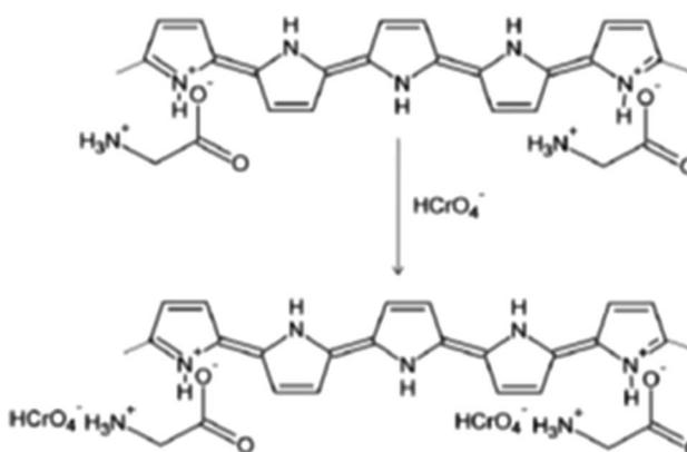
Scheme 2 The plausible adsorption mechanism for the removal of Cr(II) ions using the PPy-gly adsorbent.<sup>38</sup>
