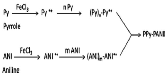
Scheme 4 The polymerization of pyrrole and aniline monomers, and the formation of PPy-PANI nanofibers.<sup>33</sup>
