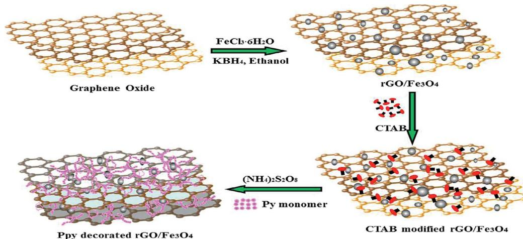
Fig. 6 Schematic of the preparation of the ternary composites.<sup>122</sup>
