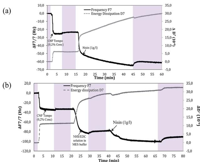
Fig. 1 Frequency and dissipation response of the 7th overtone produced by the absorption on PEI treated gold quartz sensor (a) injection of CNF Tempo (0.2%) and then nisin ( $1 \text{ g L}^{-1}$ ) (b) injection of CNF tempo (0.2%) then 2nd injection with EDC/NHS solution in MES buffer, after final injection with nisin ( $1 \text{ g L}^{-1}$ ). Pink area represents the washing after each injection with deionized water.
