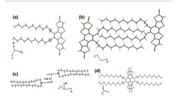
Fig. 2 Crystal structure and packing patterns of  $Br_2$ -DTmBDT: (a) crystal structure, (b) alkyl chain interdigitation and close packing, (c)  $\pi-\pi$  interactions in the dyad and (d) the top view of the dyad.
