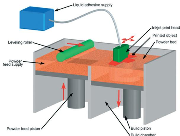
Fig. 4 Powder inkjet printing process: the roller spreads powder over the bed, with the excess powder providing a support to the printing object. Photopolymerisable ink is then deposited onto the powder to bind the particles together.<sup>20</sup> (Copyright 2008 Custom Part Net).
