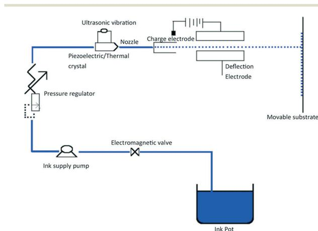
Fig. 2 Schematic illustration of DoD printing process.
